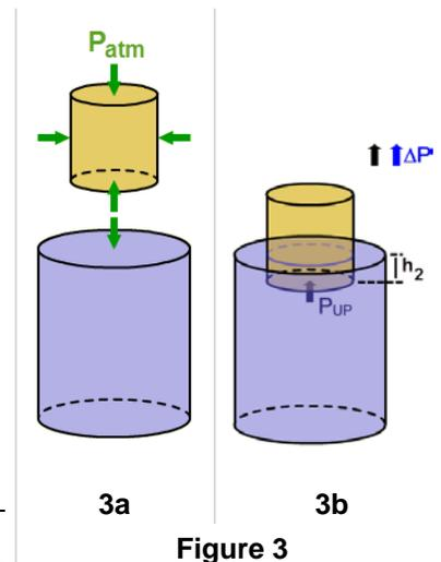
At a given depth,  $h$ , in a container of water exposed to the atmosphere there is a pressure due to the weight of the column of water above that point plus the weight of the atmosphere above the surface. This pressure is omnidirectional and given by
